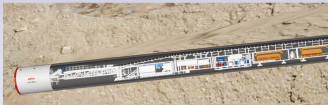
◀长距离大坡度斜井 TBM
